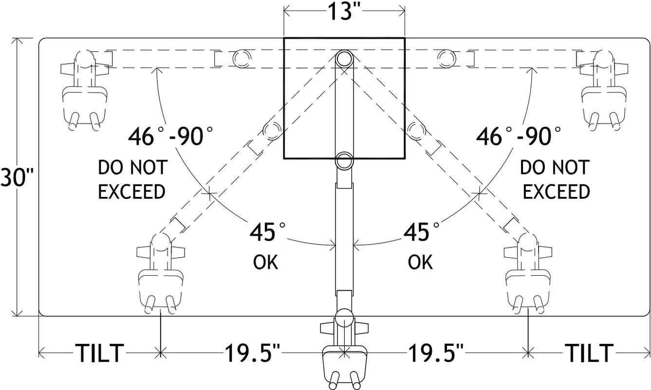
Do not swing arm exceeding 46-90 degree with full arm extended. Microscope will tilt causing injury.
